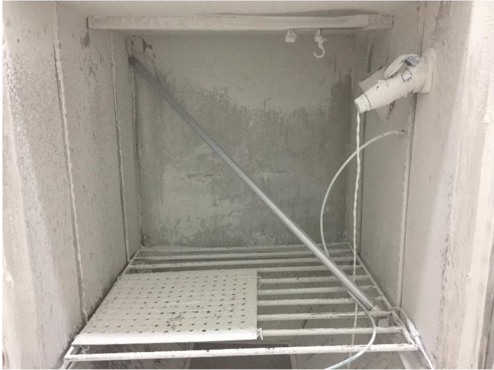
Fig.1: IP6X Before Testing
